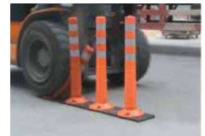
Testing by Fork Truck
